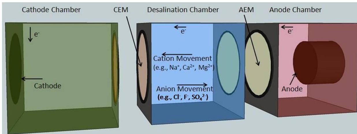
Figure 1. Schematic diagram of microbial desalination cell (MDC)
