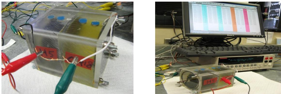
Figure 3. Pictures of experimental setup of microbial fuel cell (MFC)
