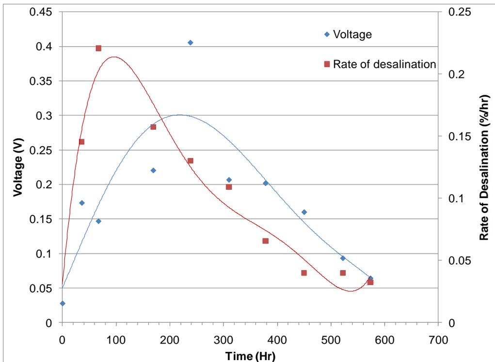
Figure 7. Rate of desalination compared to voltage output of MDC using diluted wastewater substrate
