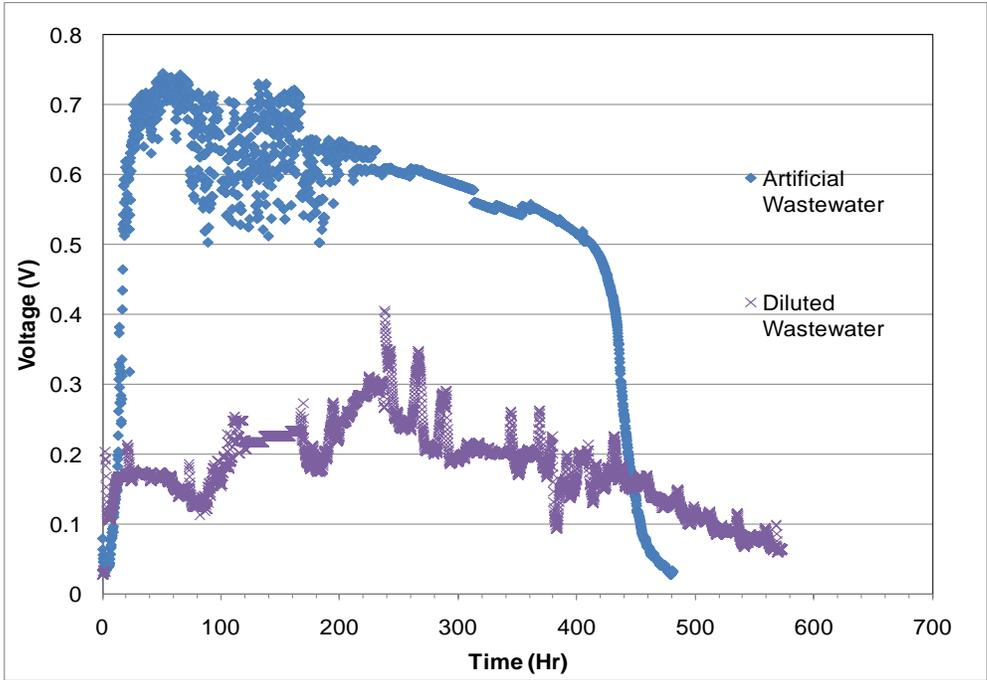
Figure 5. Comparison of energy generation of MDC with synthetic (glucose solution) and diluted wastewater
