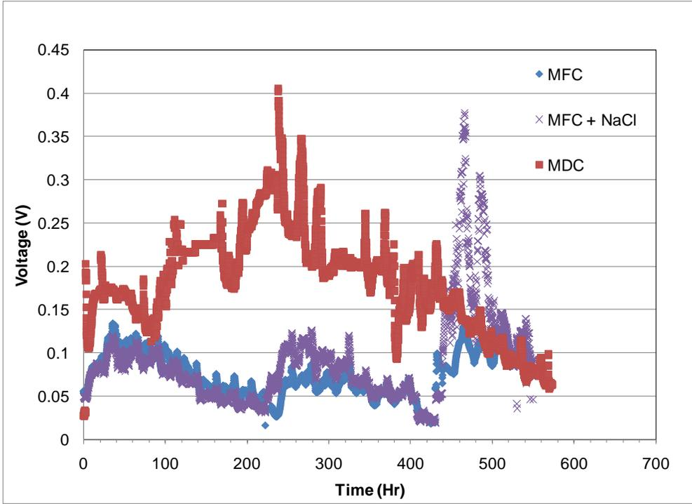
Figure 4. Energy generation of MFC versus MDC with diluted wastewater
