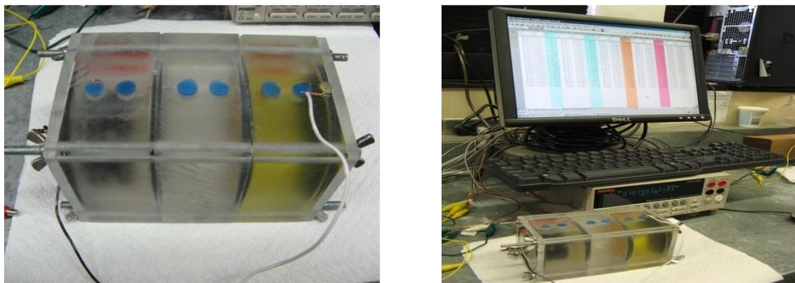
Figure 2. Pictures of experimental setup of microbial desalination cell (MDC)
